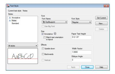
Leaving the height at 0" will allow AutoCAD to prompt you for text height while placing text in your drawing. You can check out the difference by inserting Standard style Text and the Notes style just created.
