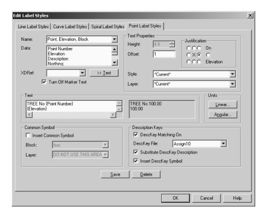
"DescKey Matching On" must be checked to allow the point label style to obtain information from the description key file. Specify the "Desckey File: " which you just created for this assignment.
