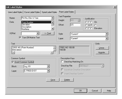
The point label style shown above will generate a point label displaying the tree number, elevation and COGO tree symbol t33 upon point(s) insertions into the drawing environment. The symbol block path is specified on the "Insert" tab of the "Point Settings" dialogue box. Point labeling must also be enabled on this tab if it is desired that LAND DESKTOP label points.
