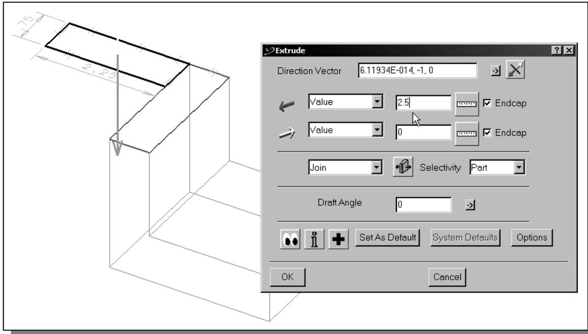
14. Click on the **OK** button to accept the settings and extrude the sketched 2D section into a 3D solid feature of the solid model.
