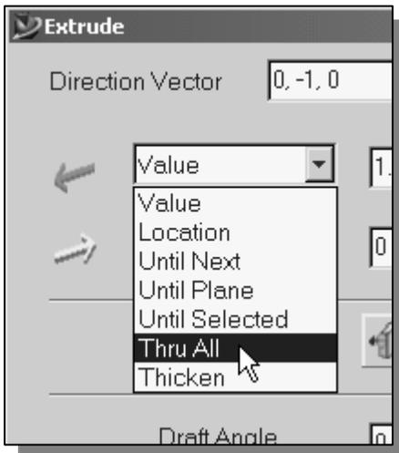
5. Click and hold down the left-mouse-button on the **depth** menu and select the **Thru All** option. *I-DEAS* will calculate the distance necessary to cut through the part.
