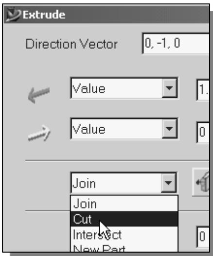
4. The *Extrude Section* window appears. Set the *extrude option* to **Cut**. Note the extrusion direction displayed in the graphics window.
