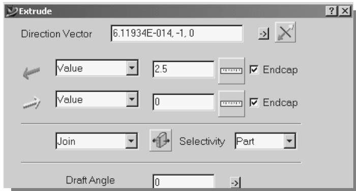
11. Enter **2.5**, in the first value box, as the *extrusion distance*.
