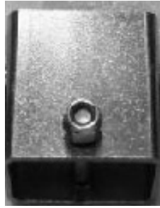
Figure 2.7: Bolt in shear and bearing
