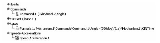
Having entered the required kinematic relation and designated the vertex on the block as the point to collect data on, we will simulate the mechanism. Click on **Simulation with**
