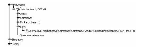
Keep in mind that our interest is to plot the position, velocity and accelerations generated by this motion. To set this up, select the **Speed and Acceleration** icon from the
