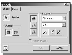
9. In the *Extrude* popup window, the **Profile** button is pressed down; *Autodesk Inventor* expects us to identify the profile to be extruded.
