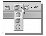
The display in the graphics window has three basic displaymodes: wireframe, shaded, and shaded with hidden edge display. To change the display mode in the active window, click on the triangle icon next to the display mode button on the *Standard* toolbar, as shown in the figure.
