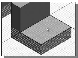
Note that the sketch plane is aligned to the selected face. *Autodesk Inventor* automatically establishes a User-Coordinate-System (UCS), and records its location with respect to the part on which it was created.
