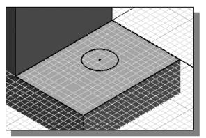
4. Create a circle of arbitrary size on the top face of the solid model as shown.
