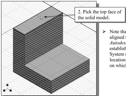
Note that the sketch plane is aligned to the selected face. Autodesk Inventor automatically establishes a User-Coordinate-System (UCS), and records its location with respect to the part on which it was created.
