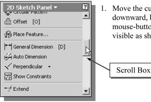
1. Move the cursor to the *Sketch* toolbar area and scroll downward, by dragging the *scroll box* with the left-mouse-button, so that the General Dimension icon is visible as shown.
