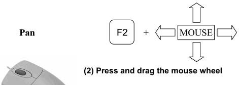
Press and drag with the mouse wheel can also reposition the display.
