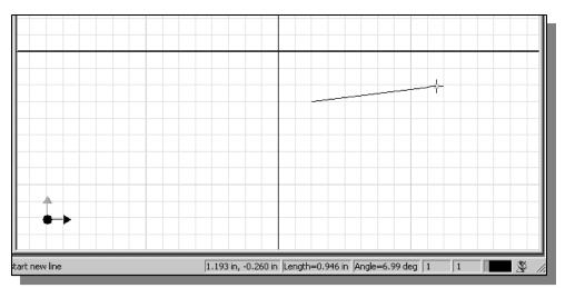
3. Move the graphics cursor toward the right side of the graphics window and create a horizontal line as shown below (**Point 2**). Notice the geometric constraint symbol, a short horizontal line, is displayed indicating the geometric property.
