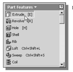
1. In the *Part Features* toolbar (the toolbar that is located to the left side of the graphics window), select the **Extrude** command by releasing the left-mouse-button on the icon.
