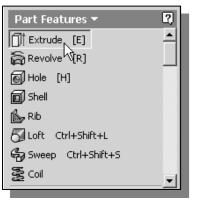
In the *Part Features* toolbar (the toolbar that is located to the left side of the graphics window), select the **Extrude** command by releasing the left-mouse-button on the icon.
