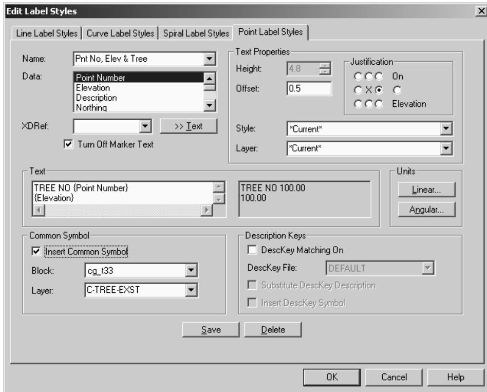
The point label style shown above will generate a point label displaying the tree number, elevation and COGO tree symbol t33 upon point(s) insertions into the drawing environment. The symbol block path is specified on the “Insert” tab of the “Point Settings” dialogue box. Point labeling must also be enabled on the “Insert” tab if it is desired that Land Desktop label points.
