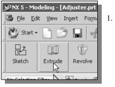
1. In the *Feature* toolbars (toolbars aligned to the right edge of the main window), select the **Extrude** icon as shown.
