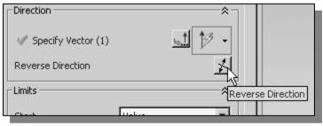
**Direction** icon to toggle the extrusion direction so that the extrusion appears as shown in the figure above.
