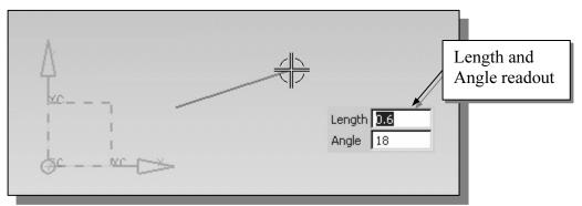
3. Move the graphics cursor directly above the previous point and create a vertical line as shown below (**Point 2**). Notice the geometric constraint symbol displayed.
