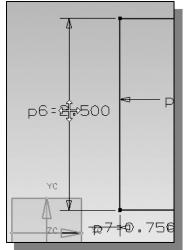
17. To reposition any of the dimensions, simply press and drag with the left-mouse-button (MB1) on the dimension as shown in the figure.
