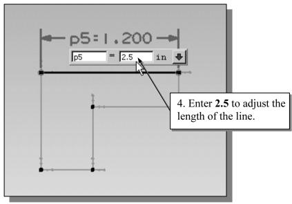
➤ UGS NX will now update the profile with the new dimension value. Note that in parametric modeling, dimensions are used as control variables.
