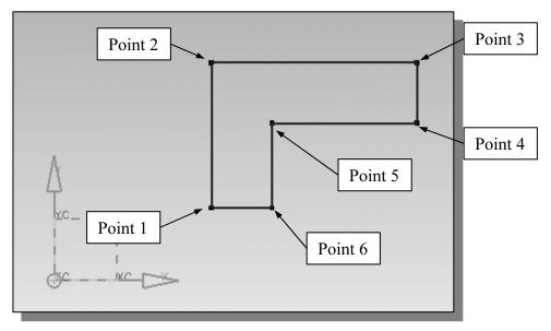
5. Inside the graphics window, click twice with the **middle-mouse-button (MB2)**, or press the [**Esc**] key once, to end the Sketch Line command.
