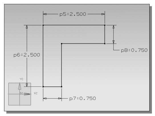
The Inferred Dimensions command is also known as the Smart Dimension command; dimensions are created based on the selection of the types and orientations of objects. You might want to read through this section again and consider the powerful implication of this command. Also consider this question: How would you create an *angle dimension* using the Inferred Dimensions command?
