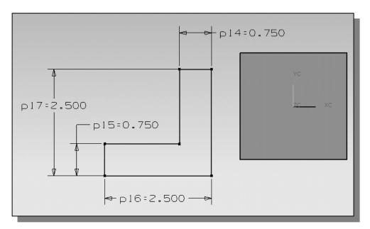
8. Create the two location dimensions to describe the position of the sketch relative to the top corner of the solid model as shown.
