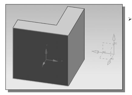
Note that the *sketch plane* is aligned to the selected face. UGS NX automatically establishes a Work Coordinate System (WCS), and records its location with respect to the part on which it was created.
