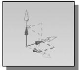
The default *sketch plane* is aligned to the *XY* plane of the work coordinate system.
