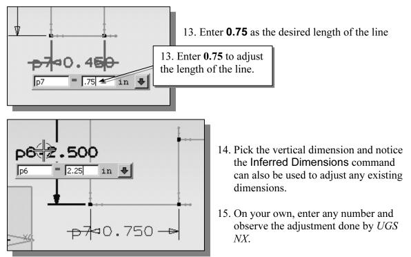
16. Inside the graphics window, click twice with the **middle-mouse-button (MB2)**, or hit the **[Esc]** key once, to end the **Inferred Dimensions** command.
