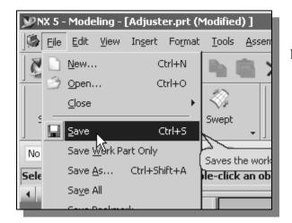
Select Save in the *File* pull-down menu, or you can also use the "Ctrl-S" combination (hold down the "Ctrl" key and hit the "S" key once) to save the part.
