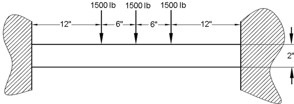
3. Use ANSYS Workbench to build a finite element model of the cantilevered beam shown below, that is made from structural steel. Determine the maximum deflection and bending stress in the beam. Then compare these values with those that you manually calculate using strength of material formulas from your textbooks (you do not have to take into account the deflection due to shear, as was done in the example problem in this chapter).
