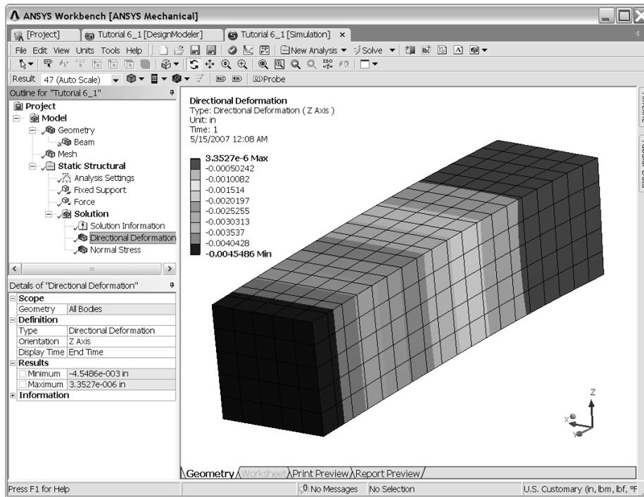
Step 12 (continued) – Note that the maximum and minimum values displayed are the range values for the contours. For example, on the **Normal Stress** plot, the red contours represent stress values ranging from 12,454. PSI to 16,012. PSI. In order to get a more precise value, use the Probe tool:
