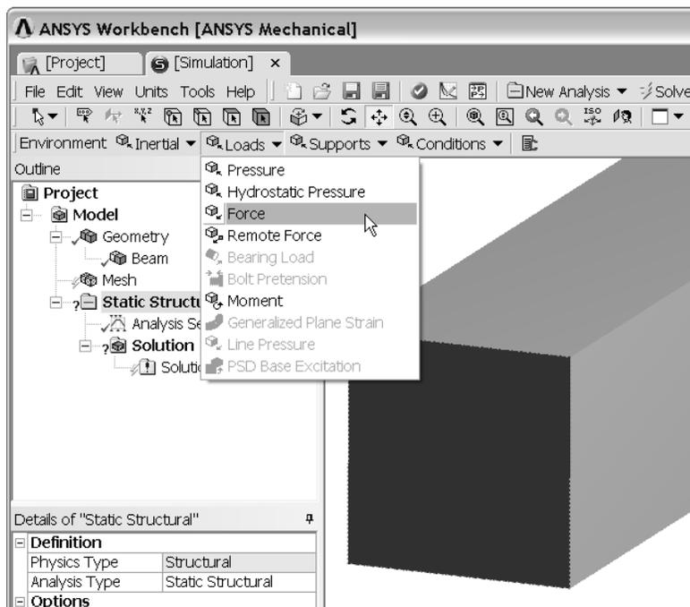
Step 8 – Set The boundary conditions. The boundary condition for this analysis consists of a fixed support at one end of the beam.
