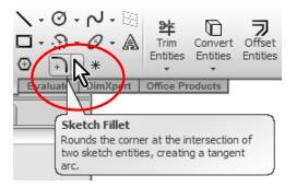
Set the fillet radius to 0.15", and click on the corners of the sketch lines as indicated to round them. After clicking on all 4 corners, click OK to finish the Sketch Fillet command. Notice that only one dimension is added. The reason is that SolidWorks adds an equal relation from each fillet to the one dimensioned fillet.
