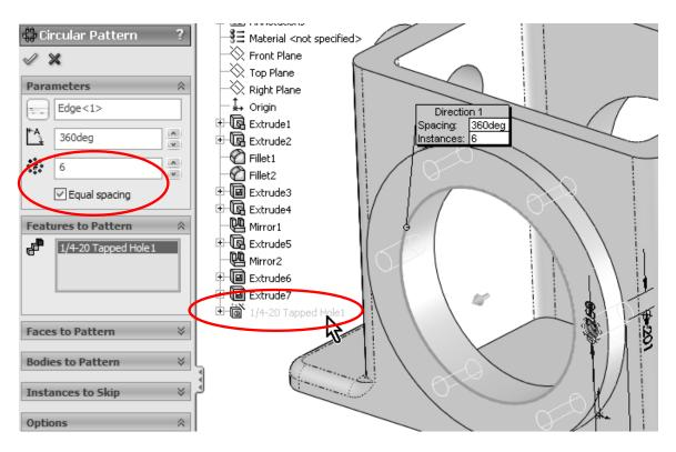
**55.** - Since we need to have the same six holes in the other side of the Housing, we will use the "Mirror" command to copy the Circular Pattern about the Front Plane to add the same holes on the other side of the housing. Review the Mirror command from steps 33 and 38 if needed. Make this mirror about the Front Plane and mirror the "CircPattern1" feature created in the previous step. After the mirror, your part should look like this:
