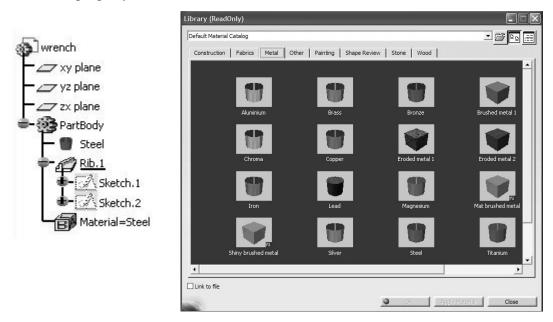
In order to inspect the values of the material properties assigned, double-click on **Steel** in the tree. It may take a minute before the database is searched. You will notice that the **Properties** box shown below opens. Choose the **Analysis** tab from this box, and the values will be displayed. Note that these values can be edited.
