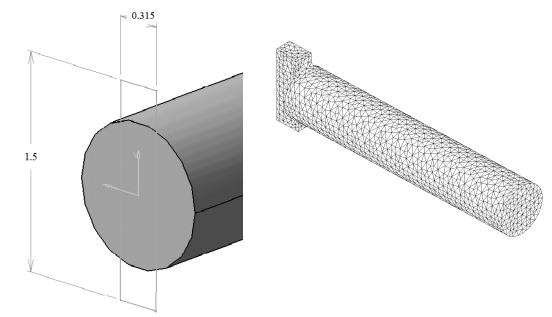
Model the part with linear solid elements with size = 0.1 and sag = 0.025 which results in the mesh shown in the previous page. Compare the hoop stress (The hoop stress is the largest principal stress "C11") with the theoretical solution from strength of materials.
