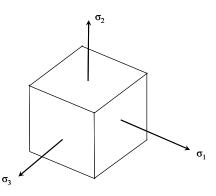
The principal stresses are postprocessed next. The principal directions are three mutually perpendicular directions along which only normal stresses act. These normal stresses are known as the principal stresses. The figure to the right displays the principal directions  $x_1$ ,  $x_2$ , and  $x_3$ , together with the principal directions  $\sigma_1$ ,  $\sigma_2$ , and  $\sigma_3$ . The standard convention in stress analysis is to label the stresses
