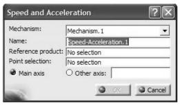
For the **Reference product**, select the **base** from the screen or the tree. For the **Point selection**, pick the vertex of the **block** as shown in the sketch below. This will set up the sensor to record the movement of the chosen point relative to the base (which is fixed).
