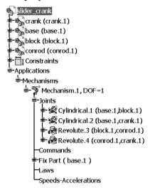
The **DOF** is 1 (if you have dof other than 1, revisit your assembly constraints to make sure they are consistent with those herein, delete your mechanism, then begin this chapter again). This remaining dof can be thought of as the position of the block along the base, or the rotation of the crank about the base. Since we want to drive the crank at constant angular speed, the latter interpretation is appropriate.
