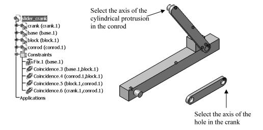
The coincidence constraint just applied removes all dof between the conrod and the crank except for rotation along the axis of coincidence and translation along that axis. To remove the unwanted translational dof, we will use a surface contact constraint (a coincidence constraint could also be applied, but we have chosen to illustrate a contact
