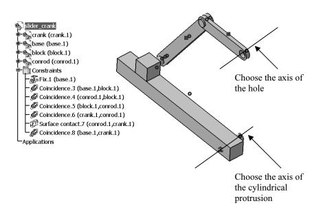
Use **Update** icon to get the final position of all parts as shown. Note that since we have chosen to create a cylindrical joint between the base and the crank, we do not need to specify a constraint to remove the translation along the axis of coincidence; that translation is effectively removed by the remainder of the assembly constraints.
