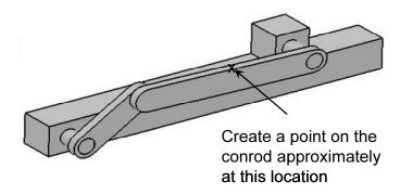
The plan is to generate two plots. The first plot is the speed of the created point against the angular position of the crank. The second plot is the acceleration of the created point against the angular position of the crank.
