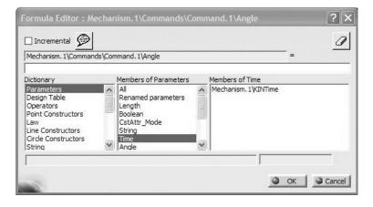
Since angle can be computed as the product of angular velocity (360deg)/(1s) in our case and time, edit the box containing the right hand side of the equality such that the formula becomes:
