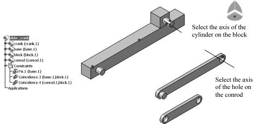
The coincidence constraint just created removes all but two dof between the conrod and the base. The two remaining dof are rotation about the axis (a desired dof) and translation along the axis (a dof we wish to remove in order to produce the desired revolute joint). To remove the translation, pick the **Coincidence** icon from the
