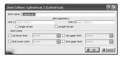
Check the **Angle driven** box. This allows you to change the limits.
