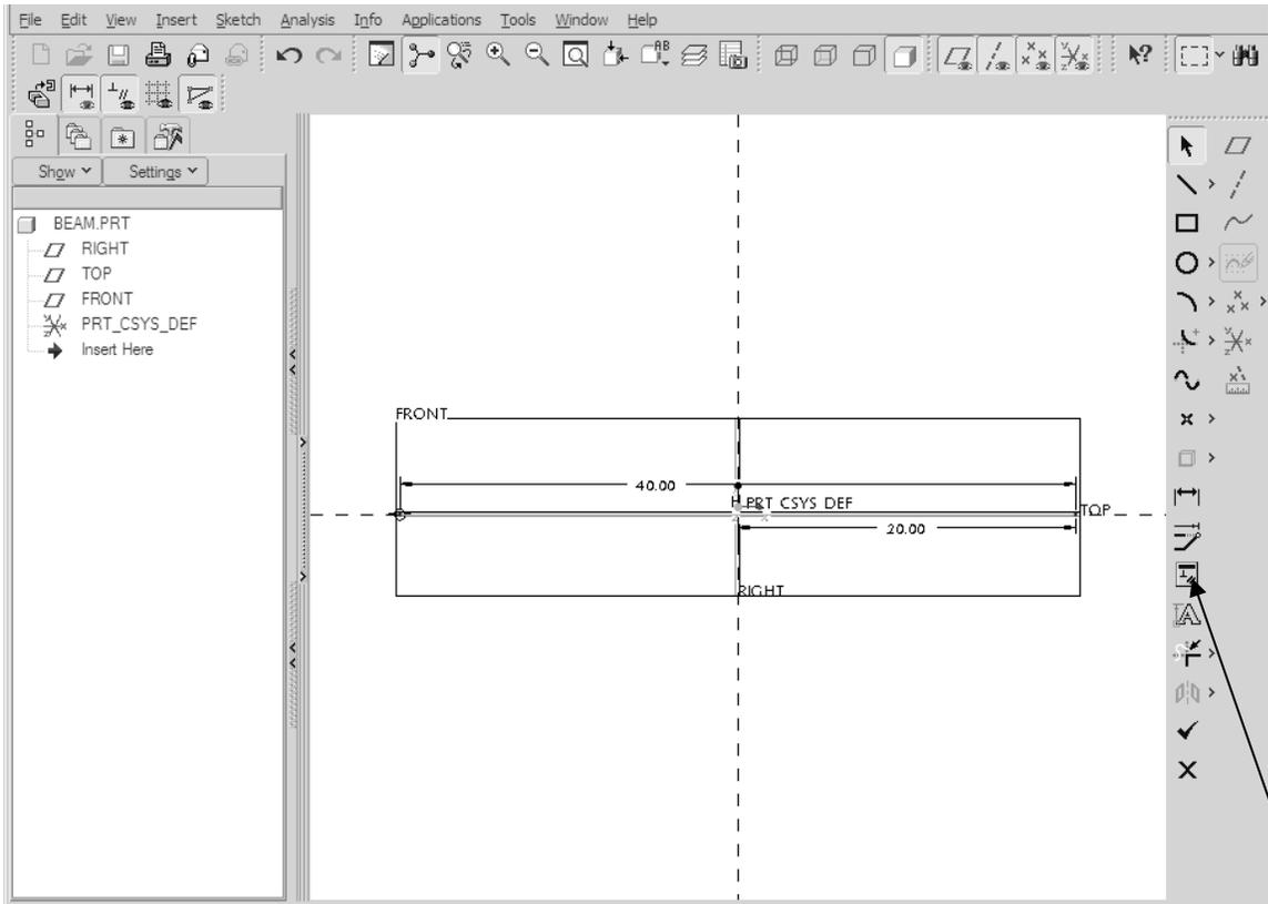
Figure 4: View of sketch for datum curve
