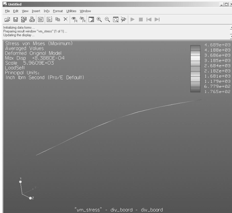
Figure 40: Von Mises Stress fringe plot for Project 1
