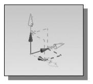
❖ Note the default sketch plane is aligned to the *XC-YC* plane of the displayed *work coordinate system*.
