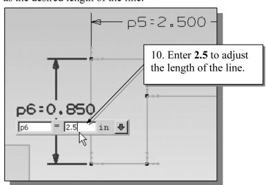
❖ When two parallel lines are selected, the Inferred Dimension command will create a dimension measuring the distance between them.
