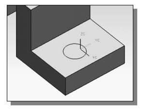
7. Create a circle of arbitrary size on the horizontal face of the solid model as shown.
