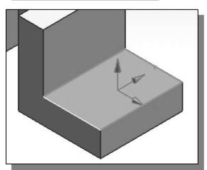
Note that the sketch plane is aligned to the selected face. *UGS NX* automatically establishes a new work coordinate system (WCS), and records its location with respect to the part on which it was created.
