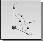
The work coordinate system (WCS) is a mobile system to assist geometric construction in different orientations. The WCS can be located and oriented anywhere in model space.
