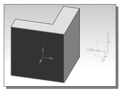
Note that the sketch plane is aligned to the selected face. *UGS NX* automatically establishes a work coordinate system (WCS), and records its location with respect to the part on which it was created.
