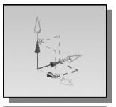
❖ The default sketch plane is aligned to the *XY* plane of the *work coordinate system*.
