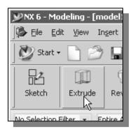
1. In the *Feature* toolbars (toolbars aligned to the right edge of the main window), select the **Extrude** icon as shown.
