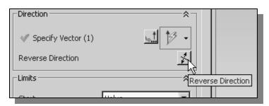
11. Click on the **Reverse Direction** icon to toggle the extrusion *Direction* so that the extrusion appears as shown in the figure.
