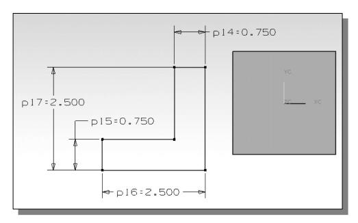
8. Create the two location dimensions to describe the position of the sketch relative to the top corner of the solid model as shown.
