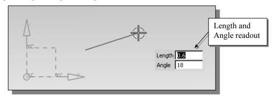
3. Move the graphics cursor directly above the previous point and create a vertical line as shown below (**Point 2**). Notice the geometric constraint symbol displayed.
