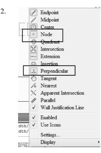
Set the Osnaps so that Node and Perpendicular are enabled.
