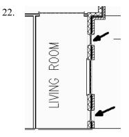
Place an **Arched Picture** window with an offset of 0" on each side of the entry door in the right living room wall.
