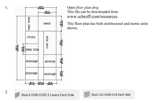
Locate the **Stud-4 GWB-0.625 2 Layers Each Side [Stud-102 GWB-018 Each Side:]** wall style on the Walls tool palette.
