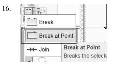
Select the **Break at Point** tool on the Break tool dropdown list to split the wall into two sections.
