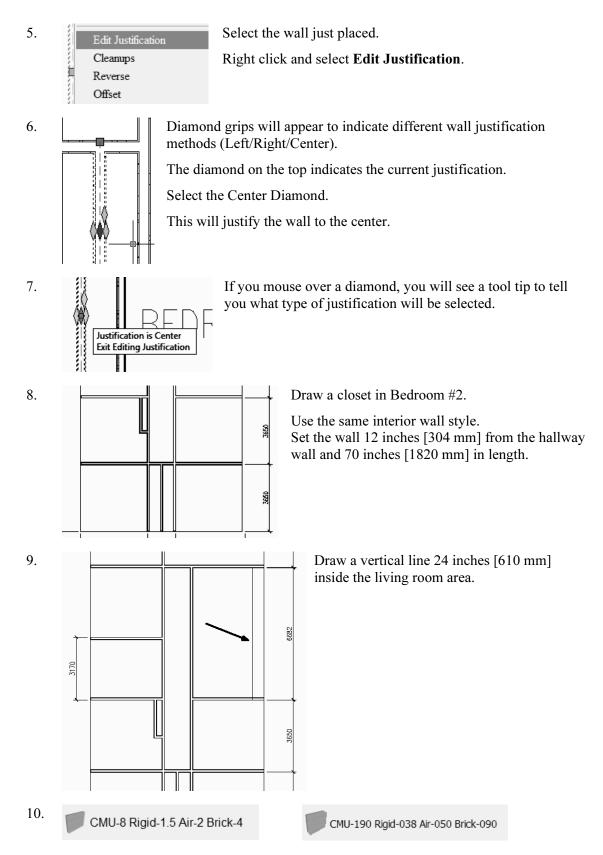
Locate the exterior wall style: CMU-8 Rigid – 1.5 Air – 2 Brick -4 [CMU-190 Rigid-038 Air-050 Brick-090].
