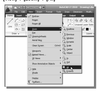
❖ The **Zoom All** command will adjust the display so that all objects in the drawing are displayed to be as large as possible. If no objects are constructed, the **Drawing** Limits are used to adjust the current viewport.
