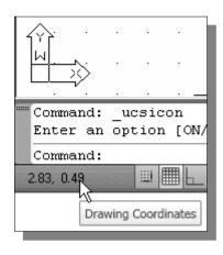
AutoCAD LT® 2010 also allows us to use absolute and relative coordinates to quickly construct objects. Absolute coordinate values are measured from the current coordinate system's origin point. Relative coordinate values are specified in relation to previous coordinates.
