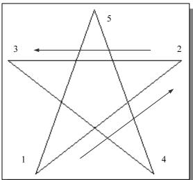
7. Repeat the above steps and complete the freehand sketch by adding three more lines (from *point 3* to *point 4*, *point 4* to *point 5*, and then connect to *point 5* back to *point 1*).
