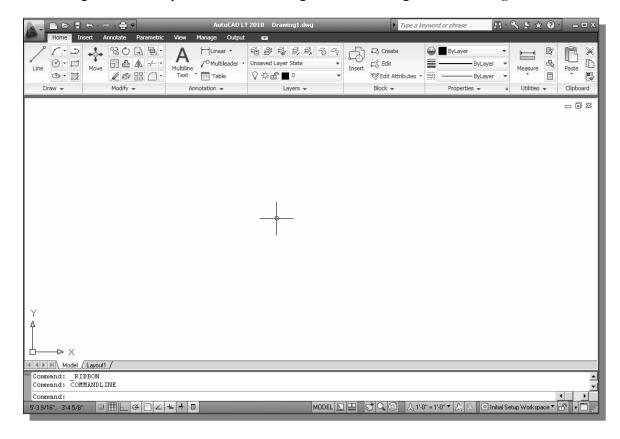
2. If necessary, click on the down-arrow in the *quick access bar* and select **Show Menu Bar** to display the **AutoCAD** *Menu Bar*. The *Menu Bar* provides access to all AutoCAD commands.
