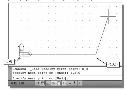
• The line we created is aligned to the bottom edge of the drawing window. Let us adjust the viewing of the line by using the Pan Realtime command.
