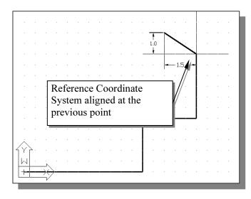
11. Using the relative rectangular coordinates entry method to create the next line, we can imagine a reference coordinate system aligned at the previous point.
