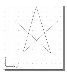
The *GRID* option creates a pattern of dots that extends over an area on the screen. Using the grid is similar to placing a sheet of grid paper under a drawing. The grid helps you align objects and visualize the distance between them. The grid is not displayed in the plotted drawing. The default grid spacing, which means the distance in between two dots on the screen, is 0.5 inches. We can see that the sketched horizontal line in the above sketch is about 5.5 inches long.
