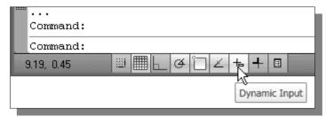
➤ The *Dynamic Input* button allows the quick toggle of the *Dynamic Input* option. We will switch *OFF* this option to discuss the basic input options available in AutoCAD LT. A more detailed discussion on this feature is presented in Chapter 2.
