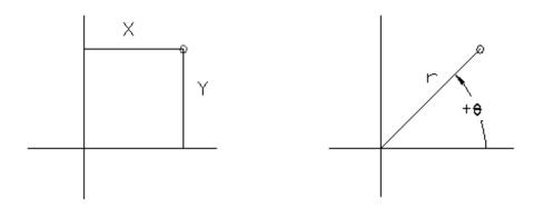
For planar geometry, the polar coordinate system is very useful for certain applications. In the polar coordinate system, points are defined in terms of a radial distance, r, from the origin and an angle,  $\theta$ , between the direction of r and the positive X-axis. The default system for measuring angles in **AutoCAD**<sup>®</sup> **LT 2010** defines positive angular values as counter-clockwise from the positive X-axis.
