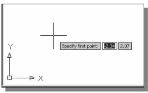
4. We will start at a location near the bottom of the graphics window. Left-click once to position the starting point of our first line.
