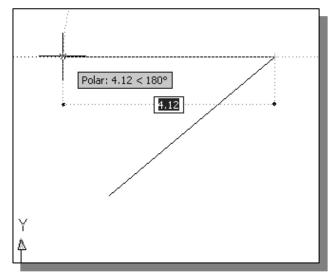
6. Move the cursor to the left of *point 2* and create a horizontal line roughly about the same length as the first line on the screen.
