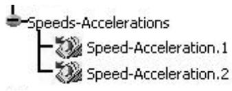
The tree indicates that **Speed-Acceleration.2** is being generated which holds the data for the point on the conrod.
