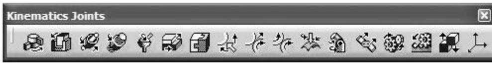
In order to animate the mechanism, you need to remove the one degree of freedom present. This will be achieved by turning **Cylindrical.2** (the joint between the base and the crank) into an **Angle driven** joint.
