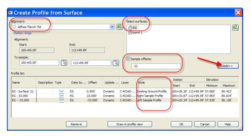
**Note:** You can also check *Sample offsets* and enter all three profile offsets at once, as shown below. Then set the *Profile Style* as required.
