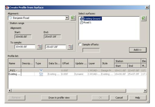
The above creates a profile along the alignment itself. If you want to sample at an offset from the alignment, select the **Sample Offsets** option and enter an offset value (negative for left), and click **Add**. You can sample multiple offsets by entering values one at a time and clicking **Add** after each.
