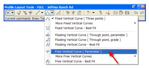
3. When prompted, pick the **first** and then **second** tangent in the profile, enter a *curve length* of **50'**, and press <Enter>.
