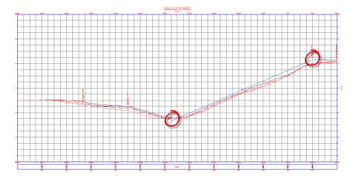
14. For the final PVI, click (Profile Station Elevation) and enter a station of **11299** and an elevation of **81.4.** When done, press Esc> and <Enter> to finish the command.
