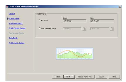
The *Station Range* second page enables you to select the station range you want to work with. Automatic includes the entire alignment's length.
