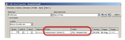
Using the styles supplied with the AutoCAD Civil 3D templates, the existing ground surface would be assigned the *Profile1* field, and the finished ground profile would be assigned the *Profile2* field.
