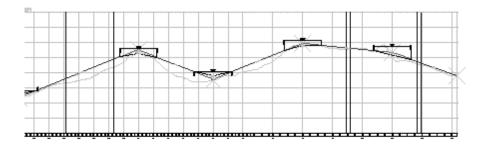
A profile is the second plane of a roadway design. It is a view of the alignment from one side of the centerline showing elevations along the alignment. An AutoCAD Civil 3D profile is a combination of a *profile view* and any number of *profiles* displayed in the view.
