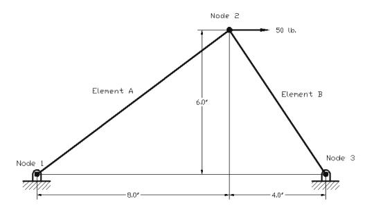
First, establish the GLOBAL stiffness matrix (system equations in matrix form) for each element.
