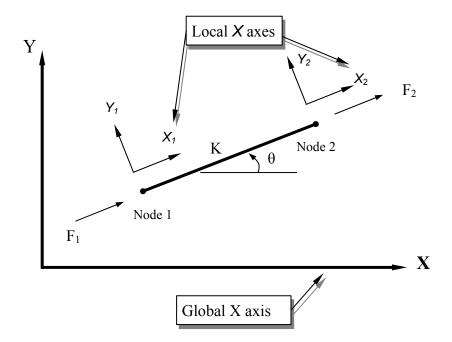
The force-displacement equations expressed in terms of components in the local XY coordinate system:
