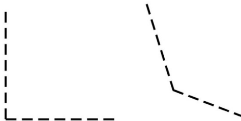
Figure 2-6: Hidden lines at corner.
