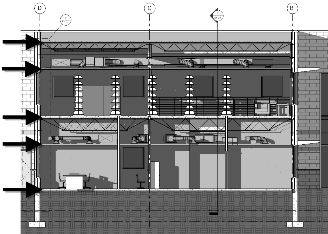
Building section showing floors, ceilings and the roof; notice structural and ductwork as well.
