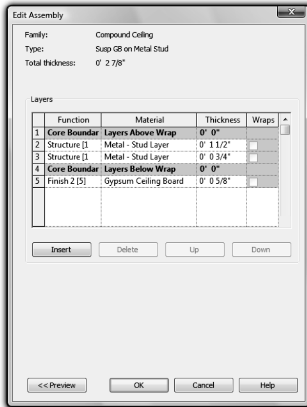
Figure 7-4.9 New ceiling – edit assembly
