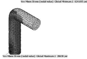
At this point we have generated two plots. The displacement and the von Mises stress contours which can be displayed individually. However, CATIA also allows you to show both plots side by side.
