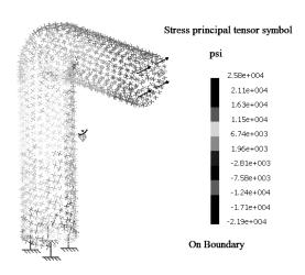
You can improve on the display of principal stresses by selecting a specific stress component to be plotted. To do so, double-click on the arrows on the screen which causes the **Image Edition**, shown to the right to open. Click on the **More** button to expand the window as shown below. Choose the **Component C11**. In CATIA, C11 represents  $\sigma_1$ , the largest principal stress.
