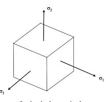
according to  $\sigma_1 \ge \sigma_2 \ge \sigma_3$ . The principal stresses are important for both theoretical reasons and practical ones. In experimental stress analysis, the positioning of strain gauges relies on the principal directions on the surface of a part.
