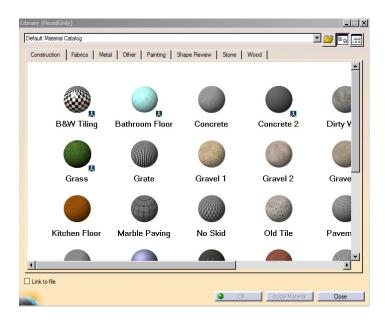
Choose the **Metal** tab on the top; select **Steel**. Use your cursor to pick the part on the screen at which time the **OK** and **Apply Material** buttons can be selected. Close the box.
