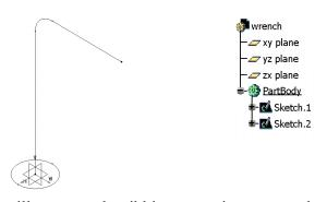
You will now use the ribbing operation to extrude the circle along the spine (path). Upon selecting the rib icon , the **Rib Definition** box opens. For **Profile** select the circle (**Sketch.1**) and for the **Center Curve** select (**Sketch.2**) as indicated. The result is the final part shown below.
