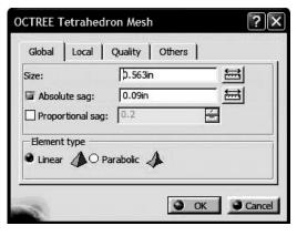
Notice that the type of the elements used (linear/parabolic) is also set in this box. Close the box by selecting **OK**.
