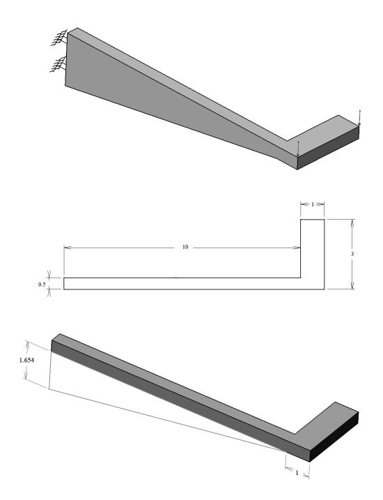
Try running the model with the two different element "size" and "sag" with both the linear and parabolic type of elements. Record the results in terms of the maximum displacement and the maximum von Mises stress in a table and comment on the results. The run time of the parabolic elements with element size of 0.1 could be substantial depending on the type of processor used.
