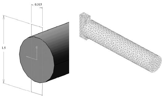
Model the part with linear solid elements with size = 0.1 and sag = 0.025 which results in the mesh shown in the previous page. Compare the hoop stress (The hoop stress is the largest principal stress "C11") with the theoretical solution from strength of materials.
