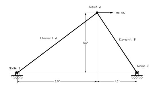
First, establish the GLOBAL stiffness matrix (system equations in matrix form) for each element.
