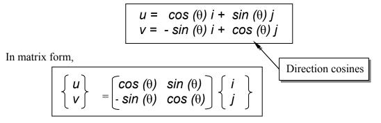
The above *direction cosines* allow us to transform vectors from the GLOBAL coordinates to the LOCAL coordinates. It is also necessary to be able to transform vectors from the LOCAL coordinates to the GLOBAL coordinates. Although it is possible to derive the LOCAL to GLOBAL transformation equations in a similar manner as demonstrated for the above equations, the *MATRIX operations* provide a slightly more elegant approach.
