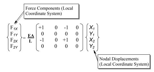
In regard to the expanded local stiffness matrix (system equations in matrix form):
