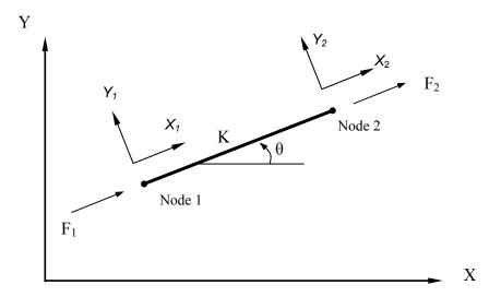
$\begin{cases} F_{1X} \\ F_{1Y} \\ F_{2X} \\ F_{2Y} \end{cases} = \begin{bmatrix} \underline{EA} \\ L \\ 0 & 0 & 0 \\ -1 & 0 & +1 & 0 \\ 0 & 0 & 0 & 0 \end{bmatrix} \begin{bmatrix} X_1 \\ Y_1 \\ X_2 \\ Y_2 \end{bmatrix}$ Local Stiffness Matrix
