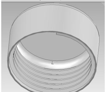
45. Select the small lip under the threads for the second surface. Make sure the Mate is Coincident and click OK twice.
