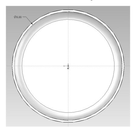
33. Exit the sketch and create a helix with a Height of 0.45, with 5 Revolutions, set the start angle to 180 degrees and turning Clockwise.
