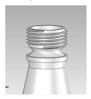
26. Create a New Part file and insert a sketch on the top plane. This will become the threaded cap for the bottle.
