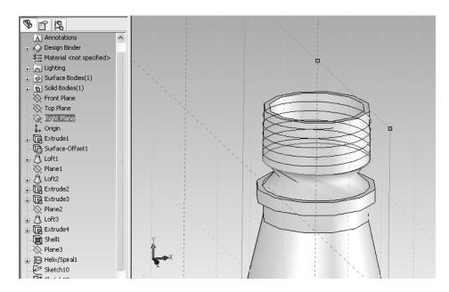
22. Look at the Right Side and zoom in to the bottom edge of the neck where the helix begins and create a sketch coincident with the bottom edge and with the dimensions as shown.
