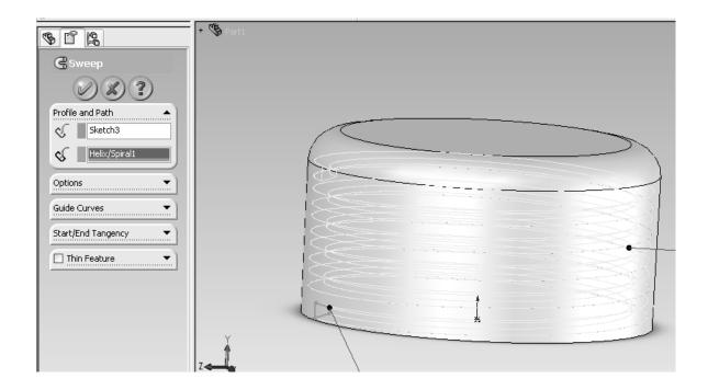
36. We now have a finished threaded cap. Now we will assemble the threaded cap and bottle together.
