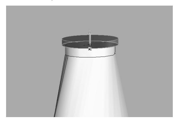
12. Draw a circle in the top surface, starting from the Origin, with a radius of 0.5in. Create an Offset Surface 0.25in away from the top surface.
