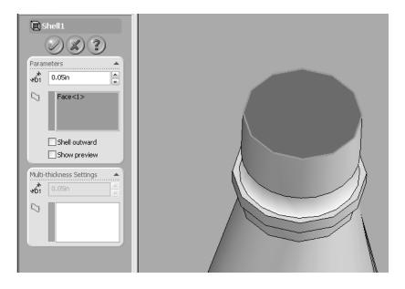
Change the Shell thickness to 0.05in. After shell, you should check if there is any lofted surface inside the bottle, if yes, you should remove it by click "Hide" as the lofted surface is used ONLY for construct the bottle.
