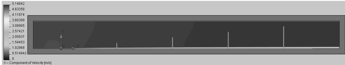
Figure 2.23b) X-velocity distribution on the flat plate.
