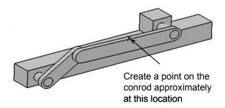
The plan is to generate two plots. The first plot is the speed of the created point against the angular position of the crank. The second plot is the acceleration of the created point against the angular position of the crank.
