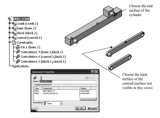
Use **Update** icon to partially position the two parts as shown below. Note that upon updating, the conrod may end up in a location which is not convenient for
