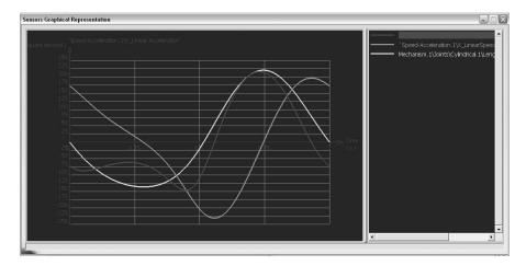
It is not uncommon that you may develop a variety of simulation results before determining exactly how to achieve the desired results. In this case, prior results stored need to be erased. To do this, click on the **History** tab History of the **Sensors** box.
