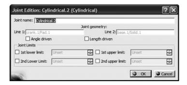
Check the **Angle driven** box. This allows you to change the limits.
