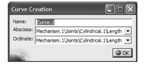
For Abscissa, select Mechanism.1\Joints\Cylindrical.2\LengthAngle For Ordinate, select Speed-Acceleration.2\LinearSpeed.
