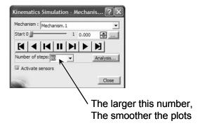
Note: If you haven't already done so, change the default units on position, velocity and acceleration to in, in/s and in/s<sup>2</sup>, respectively. This is done in the **Tools**, **Options**, **Parameters and Measures** menu shown on the next page.
