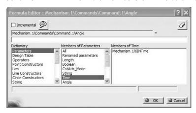
Since angle can be computed as the product of angular velocity (360deg)/(1s) in our case and time, edit the box containing the right hand side of the equality such that the formula becomes:
