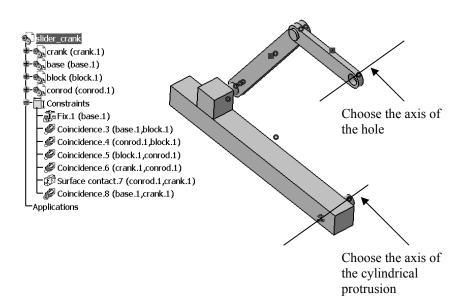
Use **Update** icon to get the final position of all parts as shown. Note that since we have chosen to create a cylindrical joint between the base and the crank, we do not need to specify a constraint to remove the translation along the axis of coincidence; that translation is effectively removed by the remainder of the assembly constraints.
