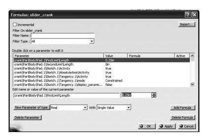
Point the cursor to the **Mechanism.1, DOF=0** branch in the tree and click. The consequence is that only parameters associated with the mechanism are displayed in the **Formulas** box.
