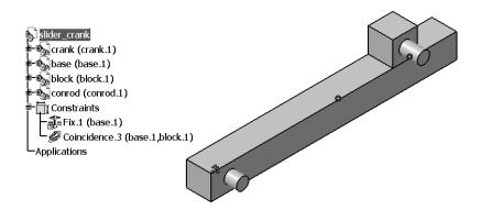
You will now impose assembly constraints between the conrod and the block. Recall that we ultimately wish to create a revolute joint between these two parts, so our assembly constraints need to remove all the dof except for rotation about the axis.
