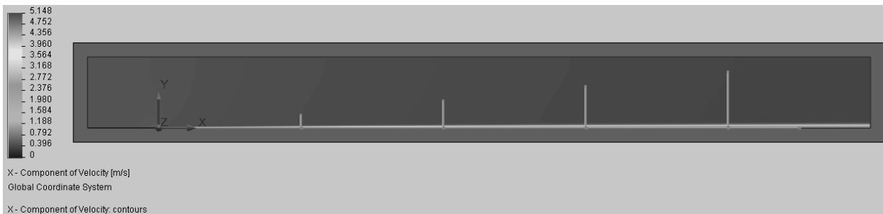
Figure 2.23b) X – Component of Velocity distribution on the flat plate.
