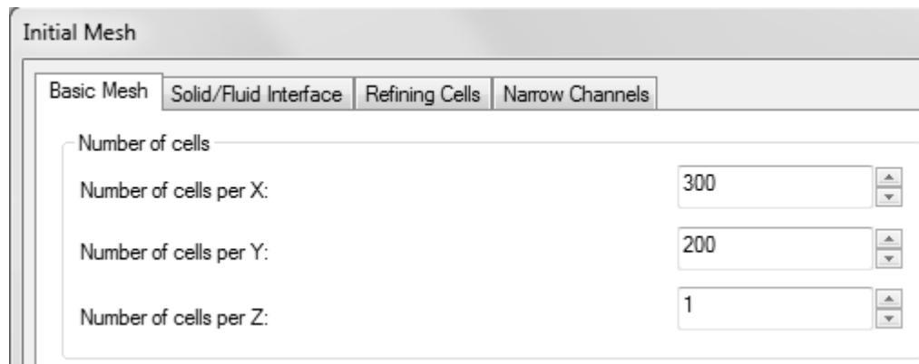
Figure 2.16b) Changing the number of cells in two directions
