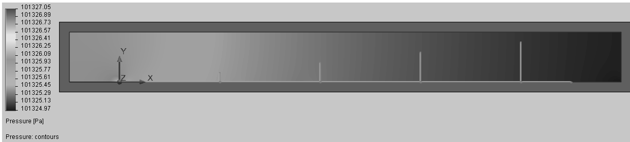
Figure 2.23a) Pressure distribution along the flat plate.
