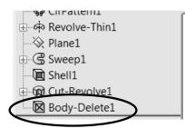
For our example we'll use the approach to select the bodies to keep at the time of making the Cut-Revolve instead of deleting the remaining bodies with an additional operation.
