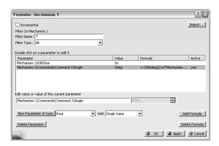
Careful attention must be given to the units when writing formulas involving the kinematic parameters. In the event that the formula has different units at the different sides of the equality you will get **Warning** messages such as the one shown below.
