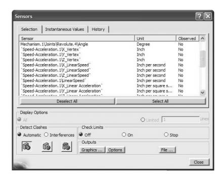
Observing that the coordinate direction of interest is X, click on the following items to record position, velocity, and acceleration of the block:
