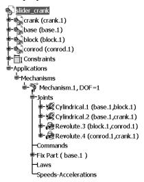
The **DOF** is 1 (if you have dof other than 1, revisit your assembly constraints to make sure they are consistent with those herein, delete your mechanism, then begin this chapter again). This remaining dof can be thought of as the position of the block along the base, or the rotation of the crank about the base. Since we want to drive the crank at constant angular speed, the latter interpretation is appropriate.
