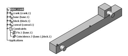
You will now impose assembly constraints between the conrod and the block. Recall that we ultimately wish to create a revolute joint between these two parts, so our assembly constraints need to remove all the dof except for rotation about the axis.
