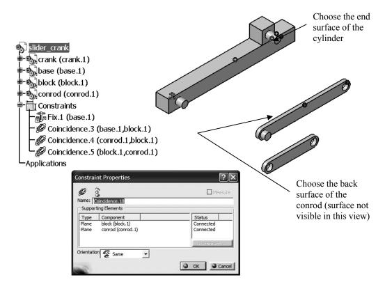
Use **Update** icon to partially position the two parts as shown below. Note that upon updating, the conrod may end up in a location which is not convenient for the rest of the assembly. In this situation the **Manipulation** icon can be used to
