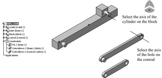
The coincidence constraint just created removes all but two dof between the conrod and the base. The two remaining dof are rotation about the axis (a desired dof) and translation along the axis (a dof we wish to remove in order to produce the desired revolute joint). To remove the translation, pick the **Coincidence** icon from the **Constraints** toolbar and select the surfaces shown on the next page. If your parts are
