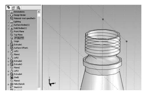
24. Look at the Right Side and zoom in to the bottom edge of the neck where the helix begins and create a sketch coincident with the bottom edge and with the dimensions as shown.
