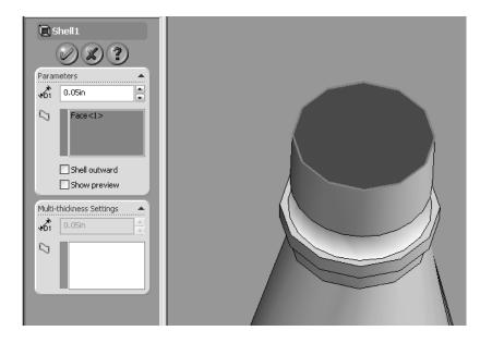
17. Change the Shell thickness to 0.05in. After shell, you should check if there is any lofted surface inside the bottle, if yes, you should remove it by click "Hide" as the lofted surface is used ONLY for construct the bottle.
