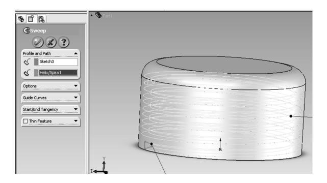
38. We now have a finished threaded cap. Now we will assemble the threaded cap and bottle together.
