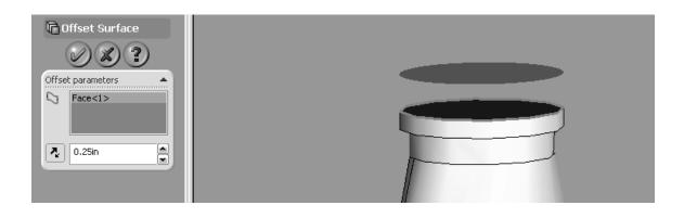
14. Draw a circle on this new surface, starting from the Origin, with a radius of .4875in. Use the Lofted Boss/Base tool to connect these two circles.
