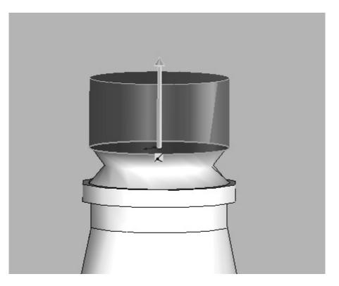
16. The body of the bottle is now complete! The final step to finish it off is to make the bottle hollow. Click on the Shell tool.
