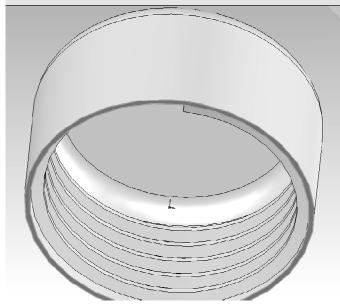
47. Select the small lip under the threads for the second surface. Make sure the Mate is Coincident and click OK twice.
