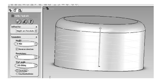
36. Create a new sketch on the Right Plane and zoom in to the bottom edge of the cap where the helix begins and create a sketch coincident with the bottom edge and with the dimensions as shown.
