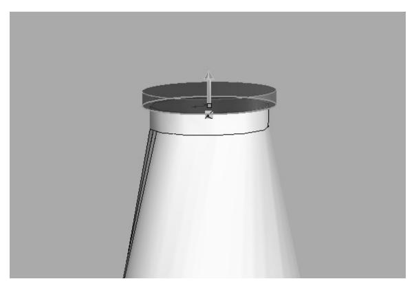
13. Draw a circle in the top surface, starting from the Origin, with a radius of 0.5in. Create an Offset Surface 0.25in away from the top surface.
