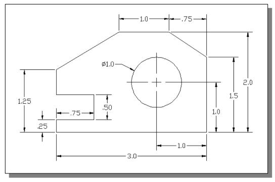
1. Inclined Support (Thickness: .5)
