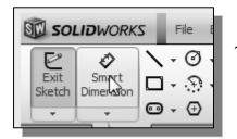
7. Select the **Smart Dimension** command in the *Sketch* toolbar. The **Smart Dimension** command allows us to quickly create and modify dimensions.
