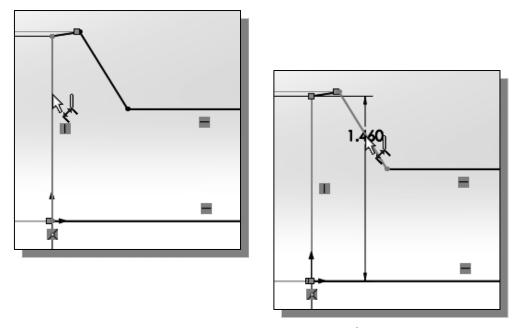
19. Select the longer inclined line on the left as the 2<sup>nd</sup> geometry to dimension.
