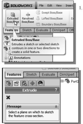
1. In the *Features* toolbar select the **Extruded Boss/Base** command by clicking once with the left-mouse-button on the icon.
