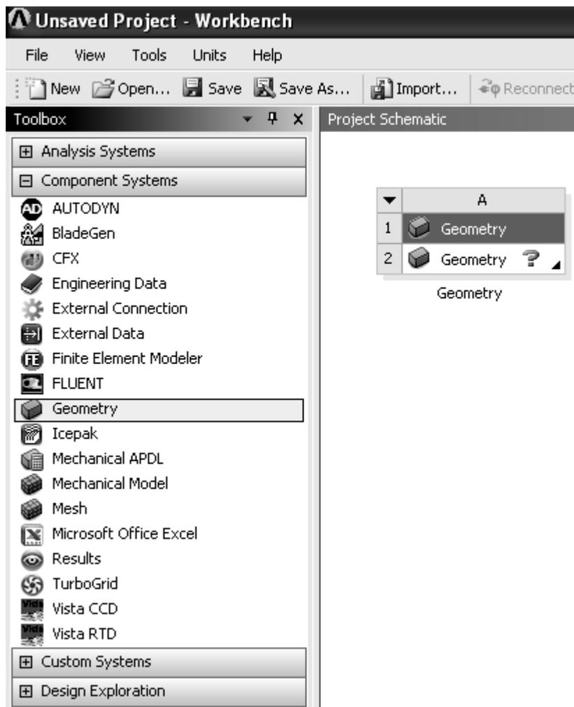
**Figure 1-2** Design Modeler in the Project Schematic.
