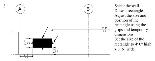
Position the rectangle 5' 6" to the right of the A grid and 3' 0" above Level 1. 4.
