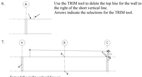
Extend the right vertical line up. Draw a new slanted line to close the profile. Set the angle to **91°**.
