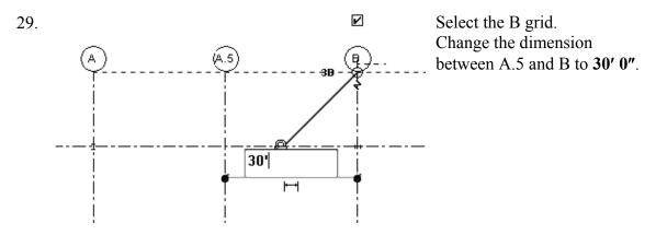
Note that the columns remain aligned to the grid.
