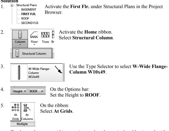
To place columns at grid intersections, select the vertical and horizontal grid.
