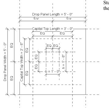
Study the parameters assigned to the different dimensions.
