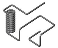
A 3D sketch normally consists of lines and arcs in series and Splines. You can use a 3D sketch as a sweep path, as a guide curve for a loft or sweep, a centerline for a loft, or as one of the key entities in a routing system.
