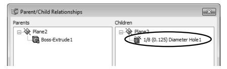
The most likely reason why the "1/8 (0.125) Diameter Hole1" feature is a child to Plane2 is that it was probably made in Plane2. We can find out in which plane or face a sketch is made by editing the sketch plane; to do this expand the Hole Wizard feature, select the first sketch (Sketch12) which is the hole's location sketch, and from the pop-up menu select "Edit Sketch Plane." Since Plane2 is listed it confirms it as the current sketch plane.
