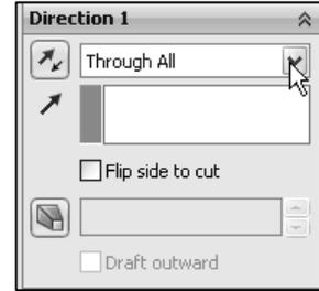
**110)** Select **Through All** for End Condition in Direction 1. The direction arrow points to the right. Accept the default conditions.
