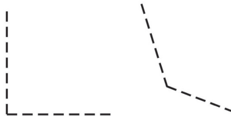
Figure 2.6-2: Hidden lines at corner.
