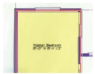
Use the FILLET command to create corners between the vertical and horizontal walls.
