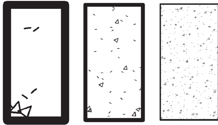
FIGURE 4-2.9 Drafting patterns automatically adjust size with view scale
