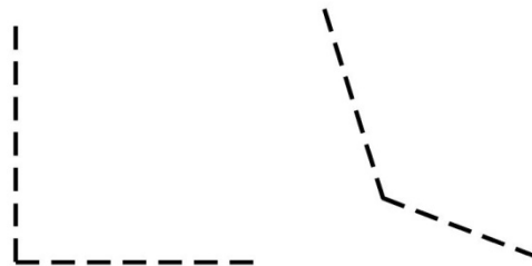
Figure 2.6-2: Hidden lines at corner.
