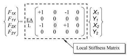
The force-displacement equations (in the local coordinate system) can be expressed as:
