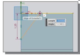
5. Place the second point aligned to and below the mid-point of the left edge as shown.
