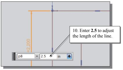
When two parallel lines are selected, the Rapid Dimension command will create a dimension measuring the distance between them.
