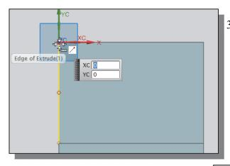
3. Use the **Profile** command and start the first line segment at the top left corner as shown.
