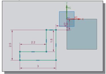
• Note that since we did not modify the **Sketch Settings**, both the *Constraints* and *dimensions* are automatically applied to the sketch.
