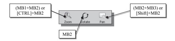
1. On your own, use the dynamic Zoom and Pan options by the mouse buttons to reposition the sketch near the center of the screen.
