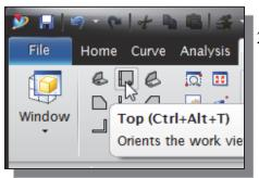
2. Select **Top View** in the **View** toolbar to change the display to the top view. (Note that the [**Ctrl+Alt+T**] key can also be used to activate this command.)
