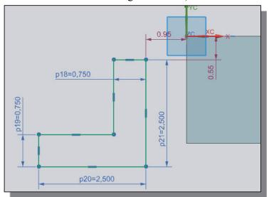
6. Modify the two location dimensions to **0.0**, this will align the position of the sketch relative to the top corner of the solid model as shown.
