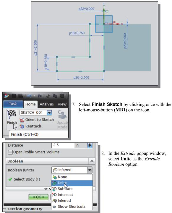
The Unite option will ADD the new feature to the existing solid. Note that the default option was set to Inferred, which means NX will determine the option based on the type of sketches created.
