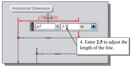
> *NX* will now update the profile with the new dimension value. Note that in parametric modeling, dimensions are used as **control variables**.
