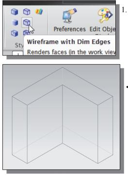
1. Pick the **Wireframe with Dim Edges** option as shown in the figure.
