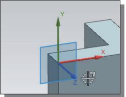
Note that the sketch plane is aligned to the selected face. *NX* automatically establishes a Work-Coordinate-System (WCS), and records its location with respect to the part on which it was created.
