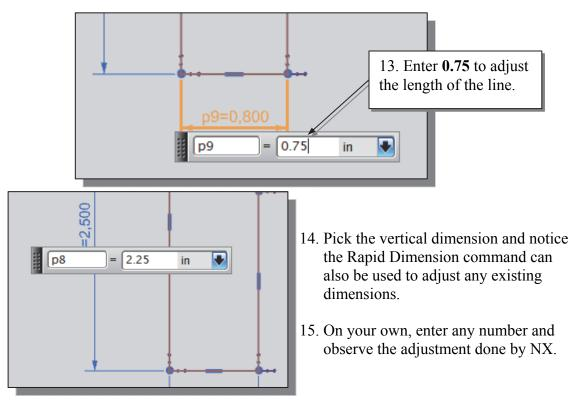
Inside the graphics window, click once with the middle-mouse-button (MB2), or hit the [Esc] key once, to end the Rapid Dimension command.
