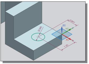
6. On your own, modify the dimensions of the sketch as shown in the figure. (Hint: there are two locational dimensions and one size dimension.)
