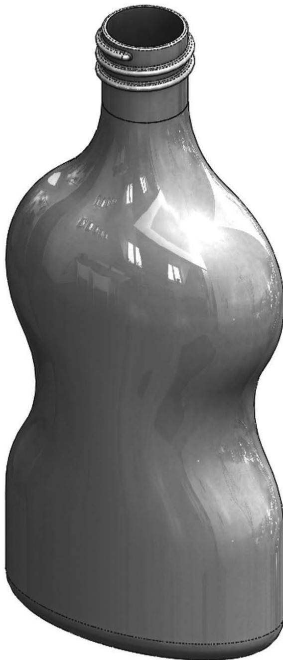
In this model we'll use two sweep features, one for the body and one for the thread. For the body we'll make a sweep with two guide curves, so we need to make four sketches: Path, Guide Curve 1, Guide Curve 2 and Profile, in that order. The reason to make the Profile last is that it has to pierce the Path and both Guide Curves for the sweep to work as expected.
