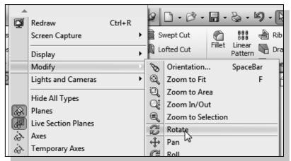
2. Move the cursor inside the graphics area. Press down the left-mouse-button and drag in an arbitrary direction; the **Rotate View** command allows us to freely rotate the solid model.
