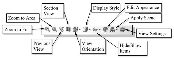
**Zoom to Fit** – Adjusts the view so that all items on the screen fit inside the graphics window.
