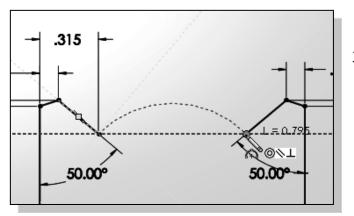
3. Select the endpoint of the longer inclined line on the right as shown.
