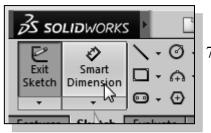
7. Select the **Smart Dimension** command in the *Sketch* toolbar. The **Smart Dimension** command allows us to quickly create and modify dimensions.
