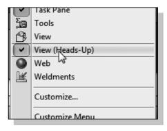
The *Heads-up View* toolbar can be customized to contain icons for user-preferred view options. **Right-click** anywhere on the *Heads-up View* toolbar to reveal the display menu option list. Click on the **View (Heads-up)** icon to turn *OFF* the display of the toolbar. Notice the **Customize** option is also available to add/remove different icons.
