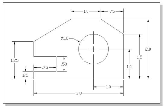
1. Inclined Support (Thickness: .5)
