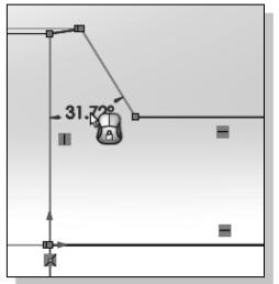
20. Place the angular dimension in the middle of the two selected lines as shown.
