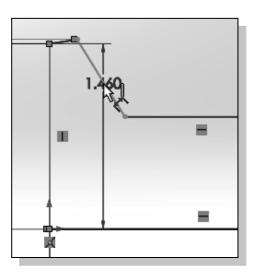
19. Select the longer inclined line on the left as the 2<sup>nd</sup> geometry to dimension.
