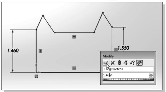
The Smart Dimension command will create a length dimension if a single line is selected.
