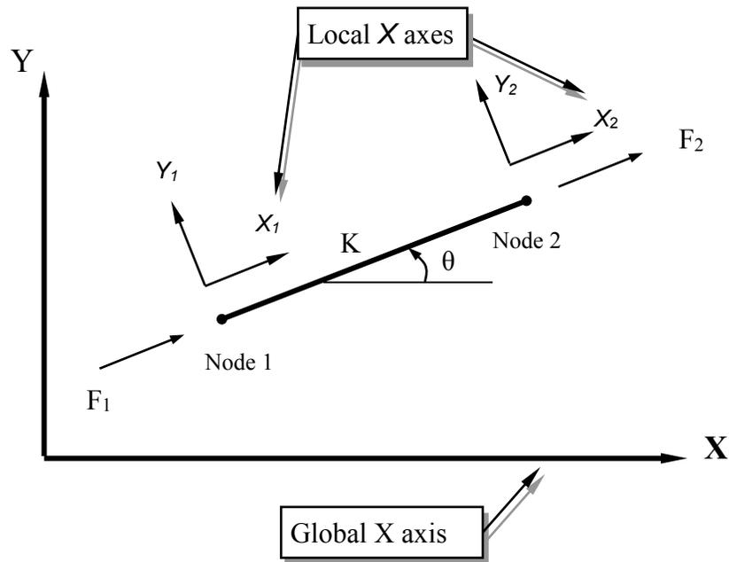
The force-displacement equations expressed in terms of components in the local  $\mathbf{XY}$  coordinate system:
