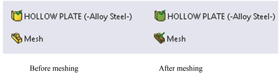
Figure 2-18: Solid and mesh folders in a Simulation study before and after meshing.
