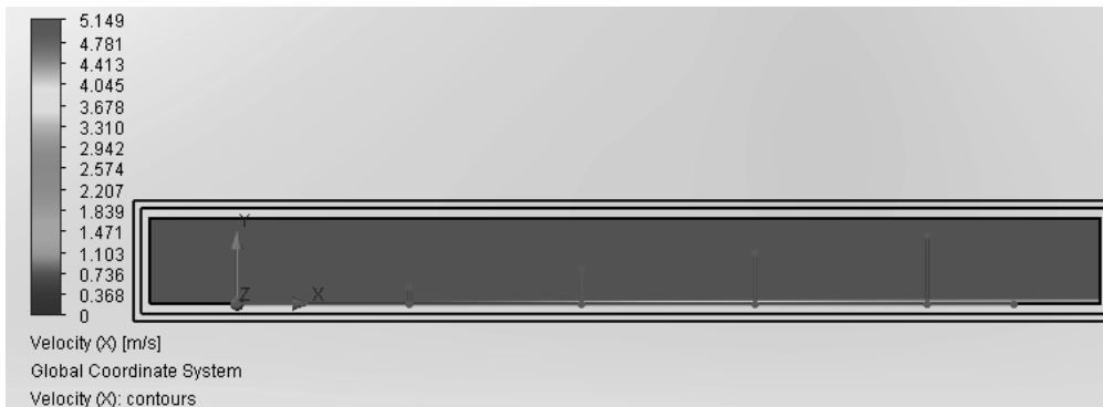
Figure 2.23b) X – Component of Velocity distribution on the flat plate
