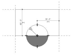
Place a cylinder at the midpoint of the bottom edge of the box.
