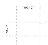
Use the ALIGNED DIMENSION tool to add dimensions to the reference planes.
