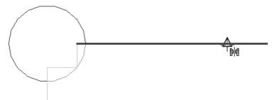
Locate the midpoint of the small horizontal line and pick.
