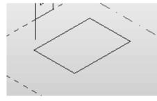
The most basic mass form is an extrude. This mass form requires a single closed polygonal sketch.
