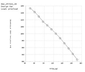
**Figure 8** Variation of Von Mises stress with fillet radius in shell model
