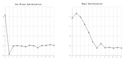
**Figure 12** Optimization history: Von Mises stress (left) and total mass (right)
