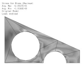
**Figure 13** Von Mises stress distribution in optimized plate
