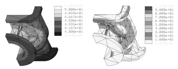
**Figure 15** Temperature distribution in the valve body (°C)
