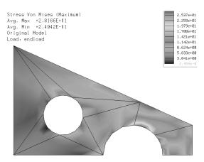
**Figure 9** Initial Von Mises stress distribution in plate before optimization
