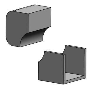
**1.10.** - Edit the "*Cut-Extrude1*" feature, turn the "Auto-select" option OFF in the "**Feature Scope**," and select the top body only. Click **OK** to finish. Now we are only cutting into the top solid, even when the cut overlaps the lower body.
