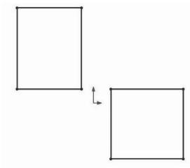
**1.2.** - Select the "Boss Extrude" command. Notice that we are not given a warning about having two separate bodies; it just works. Extrude the sketch any size that looks similar to the following image (dimensions are not important at this time) and click **OK** to finish. Making two or more extruded/revolved/swept/lofted features would work just the same.
