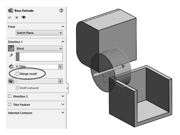
**1.7.** - After adding this extrusion we have three different bodies in our part. See how the different bodies' edges intersect each other. If the "Merge result" option had been checked, we would not see the overlapping edges as they would have merged into a single body.
